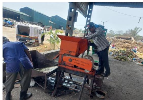
Crusher at Slurry Plant
